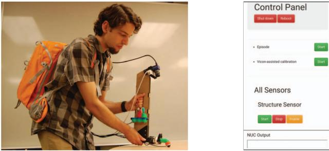
Fig. 4. Left: an experimenter holds the Proton, equipped with the OptoForce end-effector, in contact with a desk surface. Right: the mobile control interface.
